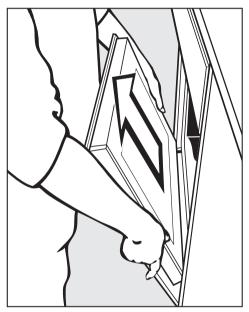
Hold the door securely at both sides and lift it upwards at an angle off the hinge guides.
